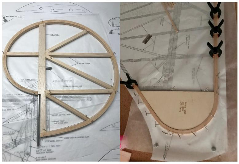
Completed rudder on the left and laminating balsa stock to create the elevator tips and trailing edges, on right. Well gang, that's about it from the building board this month (did I mention I also assembled a Proud Bird eF1 plane for our upcoming Pylon races?)
