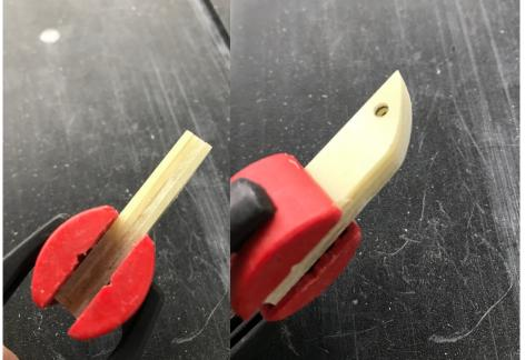
Referring to the first photo, you will notice several small holes drilled in the lower half of the horns... this is so that the epoxy used to bond them in their slots will flow into the horn material, essentially "pinning" the horns in place. I also rough up the surfaces with coarse sandpaper and clean thoroughly with alcohol before gluing them in place.
