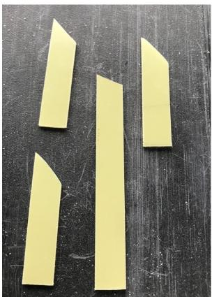
Using G10 material leftover from my Wildcat, I cut 4 pieces, 2 for each aileron. After shaping, the four pieces were clamped together and a single hole drilled through all four to accommodate a ball link bolt. Btw: this G10 is VERY hard. I have used my scroll saw to cut it, and the blades go dull very fast. Even a carbide tipped blade will show signs of dulling after a few cuts.
