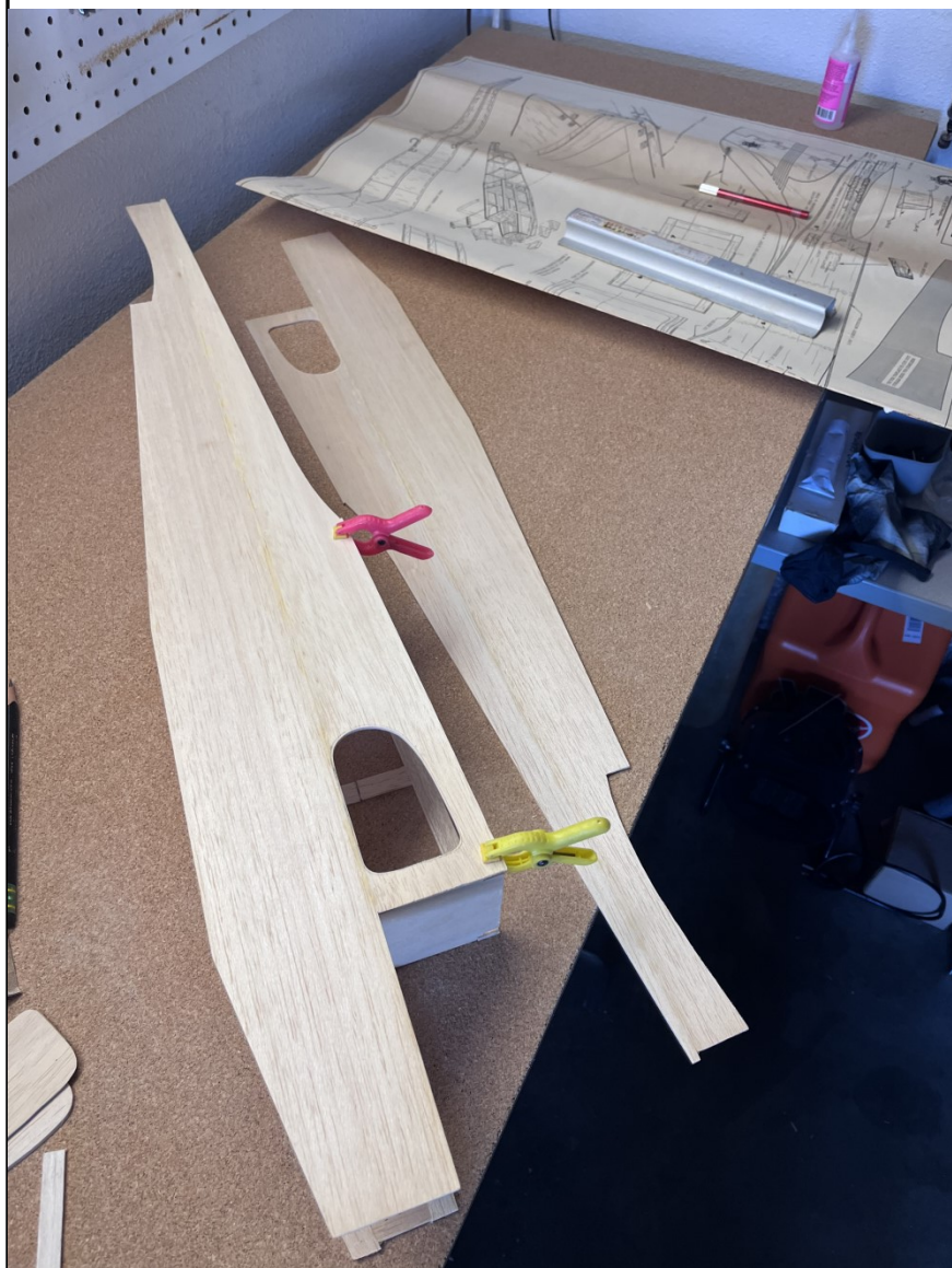
The fuselage framework is built mostly from balsa stock, with a mixture of some die cut parts. Even the fuselage sides must be cut from balsa sheeting and shaped to match the plans. This was no ARF!
