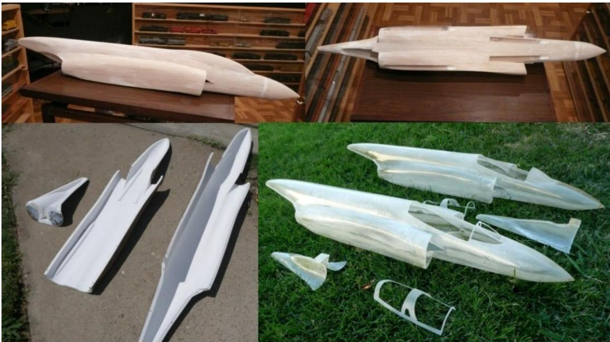
**This F-4 Phantom requires making a mold for glassing. The recessed areas for the missiles, and behind the intakes would be very difficult to sand and shape. And there would also be the problem of getting it off the plug. It takes a lot more time to make molds, but on some aircraft it is the only way to go.**
