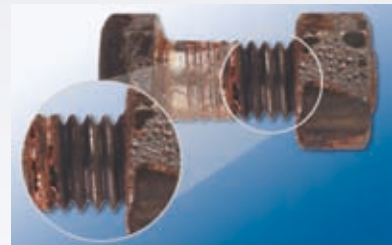
Engagement area of rusty bolt that did NOT have Loctite® threadlocker applied
