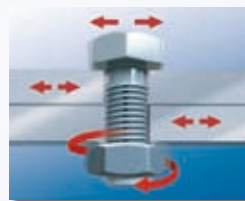
Vibration and loosening
